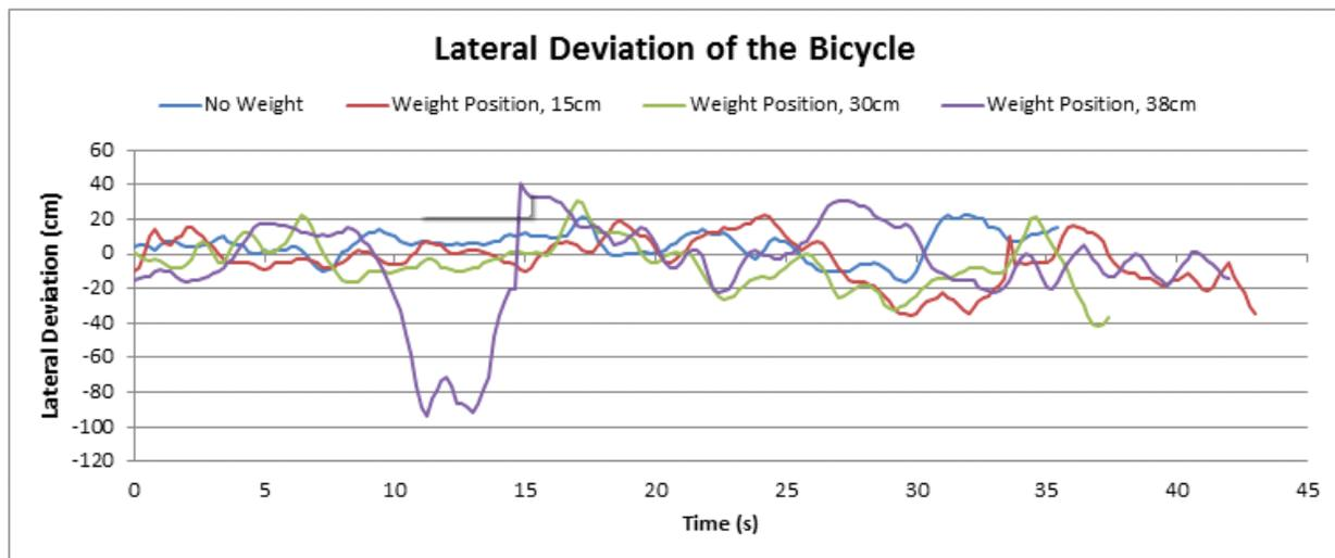
Figure 3: Measurements from downward pointing GoPro camera yielded experimental lateral deviation traces versus time
