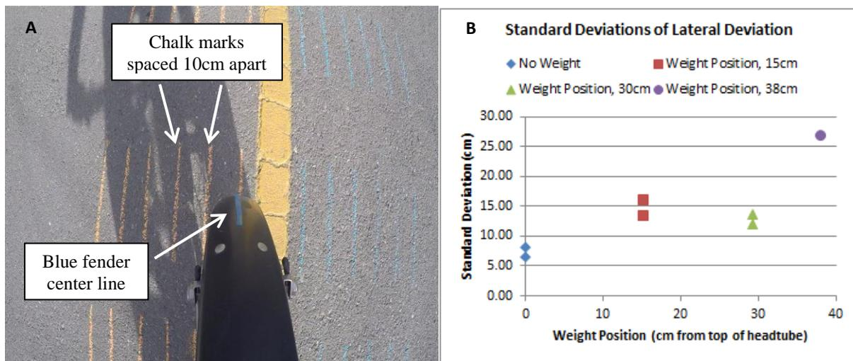
Figure 2: a) Rear wheel lateral position of blue fender center line from center of desired (yellow) tracked line was measured using a downward pointing GoPro camera yielding b) standard deviations of lateral deviation vs mass position  $d$ .
