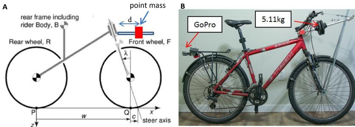
Figure 1: Theoretical and experimental bicycle schematics. Fig. 1a is adapted from [2] and depicts the idealized additional point mass. Fig. 1b shows the preliminary physical realization with a 5.11 kg mass mounted on a bar extending from the steer tube.
